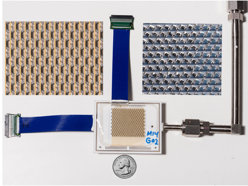
Fig. 1. Assembled detector with gas fill port, readout and high voltage feed cables. The gas feed tube connects to a shut-off valve, not shown. Left inset: cavities with readout bus lines. Right inset: array of quench resistors. Color online.
