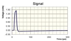
Figure 8: The time profile of the sense line signal produced by the hit cell in the multi-cell chain in Figure 6. The signal appears across the 120  $\Omega$  output impedance.
