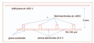
**Figure 2:** 2D side view of an initial conception of electrode geometry along one coordinate of a PPS cell. In this view the electrode layout evokes a Microstrip gas counter. The electrodes however are not long strips, but have a limited depth into the page of order hundred microns. Specified potentials are suggestive.
