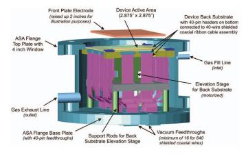
**Figure 10:** Design of PPS test vessel under construction, showing front plate (drift electrode), sectored back plate active pixel detection area, shielded coaxial ribbon signal wiring, signal feedthroughs, gas ports, motorized back plate adjustable gas gap mechanism, aperture window and chamber structure.
