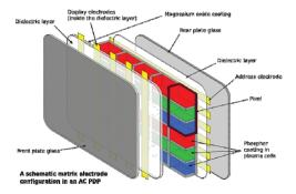
**Figure 1**: Structure of an AC type Plasma Display Panel showing the basic elements. The columnar plasma discharge region is defined by the crossing electrodes. The gas mixture comprised of noble gasses is hermetically sealed in the glass envelope. In a PPS device phosphors, MgO coatings and dielectric layers over the display electrode are absent.
