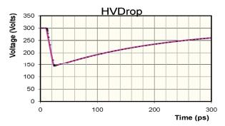
**Figure 7:** The time profile of the high voltage drop across the hit cell in the multi-cell chain in Figure 6. The rise and fall times reflect the cell capacitances and resistances. The drop to  $\frac{1}{2}$  the cell potential occurs with a (10%-90%) rise time of ~ 8 ps. The fall time (1/e return to baseline) is ~250 ps. The high voltage *across adjacent cells* remains unchanged at 300 V, indicating that the discharge remains localized.
