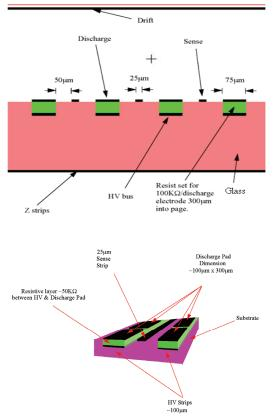
**Figure 5**: (Top) Side view of electrode configuration where embedded cell resistors derive from a resistive layer bridging between the discharge electrode and the high voltage line. The discharge electrodes are shown recessed into the substrate. (Bottom) A perspective view.
