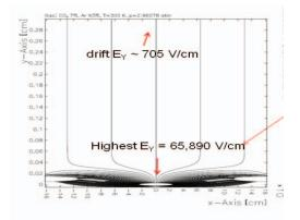
**Figure 3:** The electric fields in the drift and avalanche directions for the round electrodes of the cell represented in Figure 2 (x-axis units in  $cm^*10^{-3}$ ). The field between the avalanche and sense electrodes reaches a similar value as does the field from the drift region as it nears the sense electrode.
