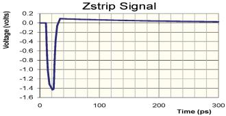
**Figure 9:** The time profile of the pulse on an orthogonal Z-strip produced by the hit cell above.
