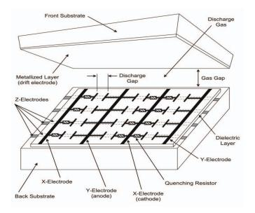
**Figure 4:** Conceptualization, not to scale, of electrode configuration of a photosensitive PPS cell. This is a 4-electrode configuration. The top plate serves as the drift field electrode. The X and Y lines define cells with embedded resistors and avalanche discharge gap regions.
