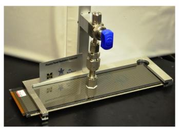
Fig. 3. PDP "refillable" test panel.
