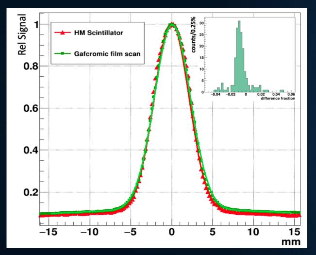
HM scintillator resolution is similar to Gafchromic film resolution (≤ 25 μm).
