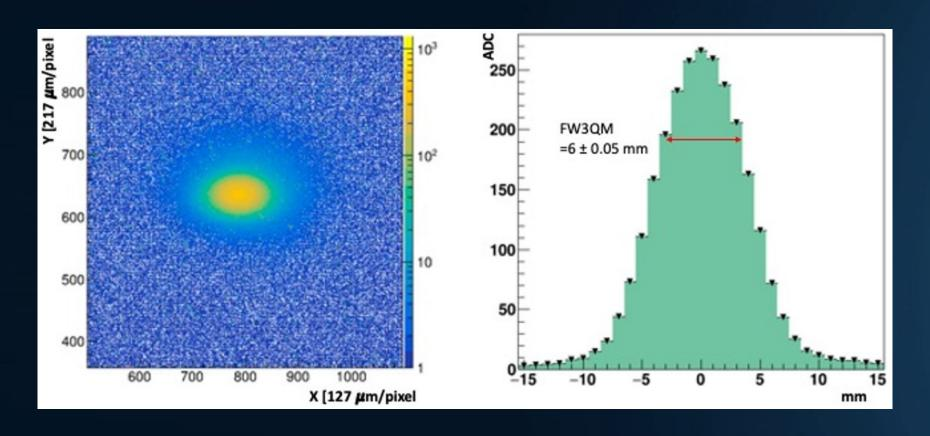
Left – Single 1 ns pulse image of **3.3 nC** electron beam (8 MeV) hitting the HM scintillator. Right – From pulse profile, dose per pulse = **7.9 Gy/pulse** (at 30 Hz) => **237 Gy/s**.
