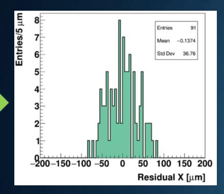
(Left) reconstructed beam centroids in pixel units plotted against precise location of a 3 mm beta source translated along the X coordinate of the FBSM. (Right) The residual distribution of the reconstructed positions yields spatial resolution of  $37 \mu m$  (RMS of fit residuals using Camera-E at 200 fps).
