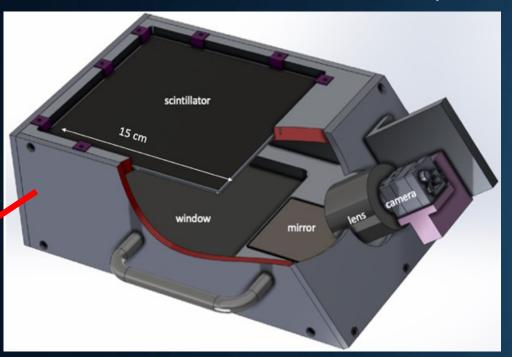
Protoype FLASH Beam Scintillator Monitor (FBSM) single camera, 15 cm x 15 cm
