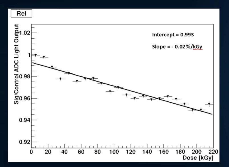
Low signal loss of ~0.02%/kGy measured over 216 kGy in 15 minutes (i.e., rate = 237 Gy/s).
