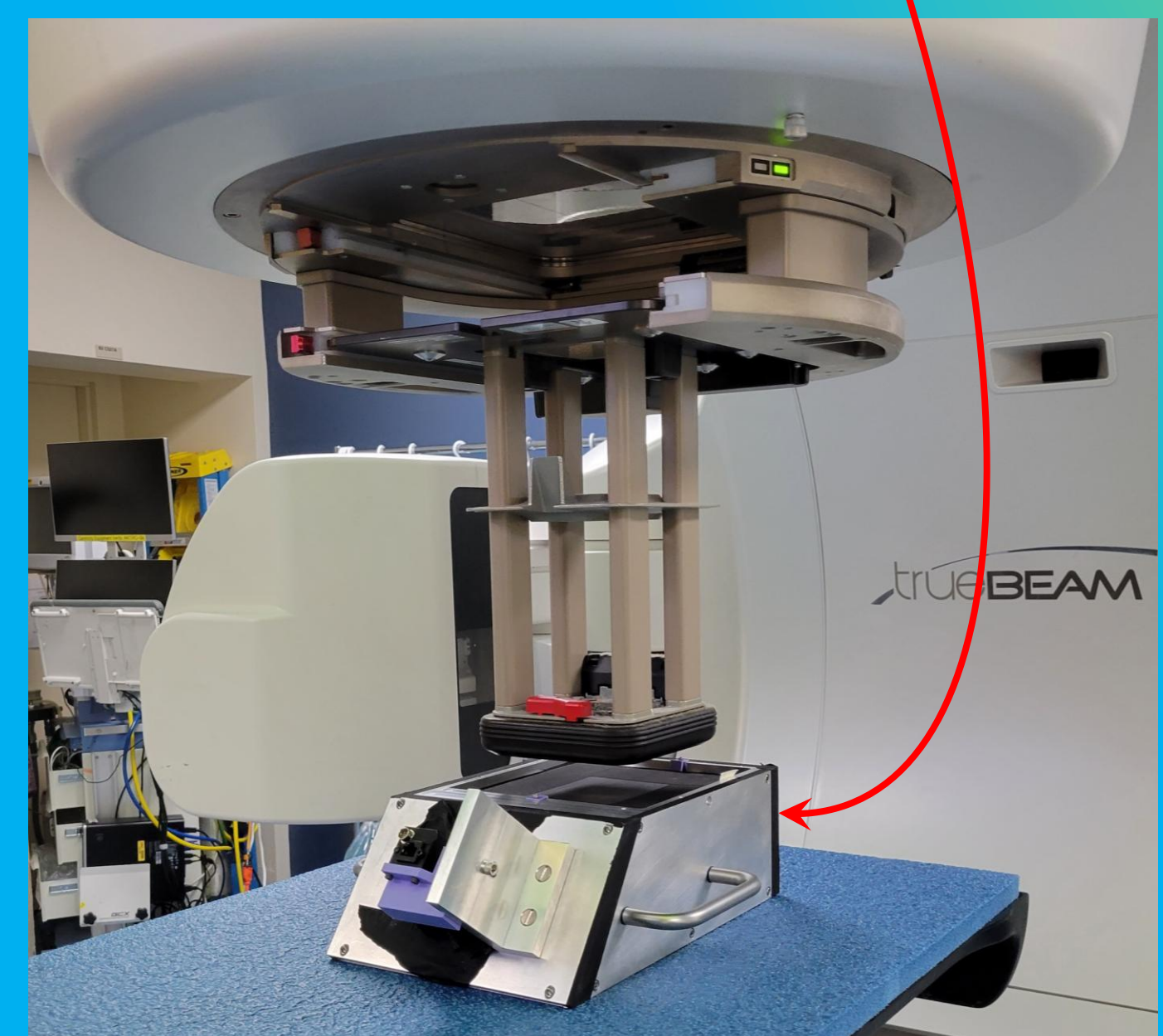
1 st Generation prototype tested with Varian 6-16 MeV electron linac at UMH.
